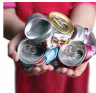
Although they're made of metal, these cans are able to be crushed rather easily. This tells us that the metal used is malleable.
